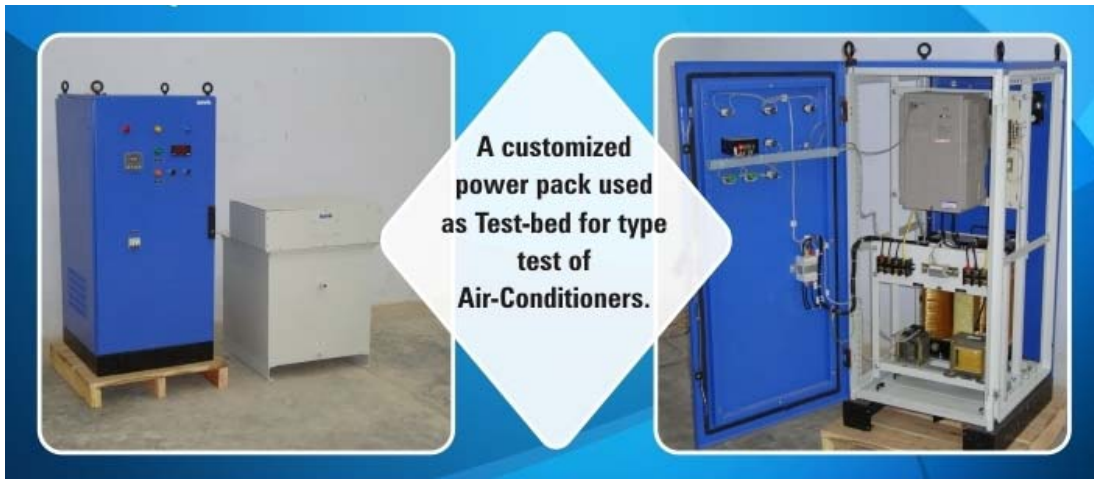
Photo showing Power Pack for Air Conditioner Test Bed
